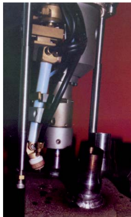
special torch for header drum stud welding
