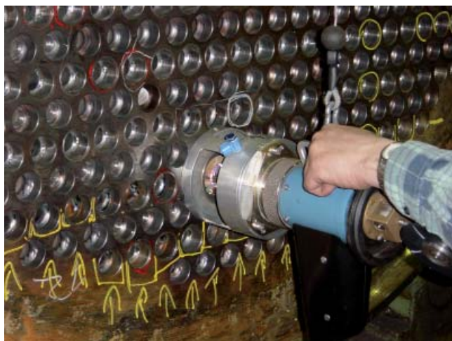
T-250 with standard double gas shield chamber
