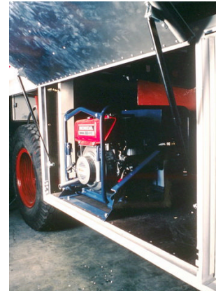
Generator and compressor in heated compartment
