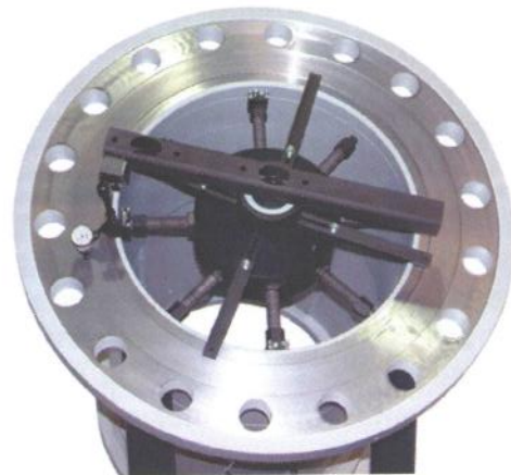
Inserting and aligning the clamping device
