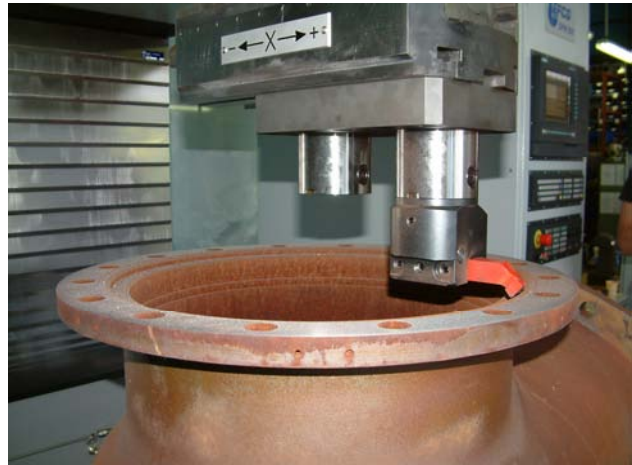
Face turning of flanges
